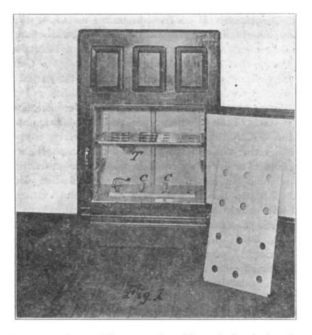
with a thermoregulator (Figs. 1 and 2, T) and circuit breaker (Fig. 2, B), from which plug connection was made to a lamp socket on a 110 a. c. circuit. A pilot light (Fig. 2, P) was also installed as indicated. The thermoregulator of the disc type was placed as shown in Fig. 1; this was selected as the best position to obtain and control the average temperature of the lower compartment. Two 1.2 cm. holes were bored
