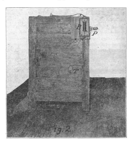
opened too frequently. Best results were obtained by keeping only one piece of ice in the ice chamber, in order to have a minimum cooling surface exposed. In ordinary weather a 15-pound piece was put in every morning, but during the hottest weather it was iced twice a day.
